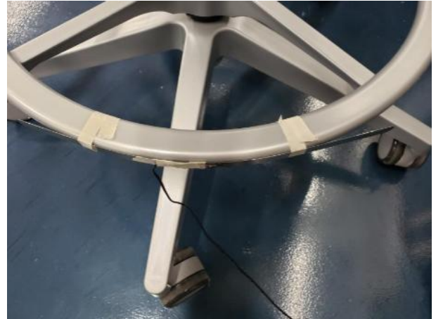
Fig. 4. The experiment apparatus of the feeler and strain gauges tightly wrapped around the laboratory stool footrest using masking tape [2].
