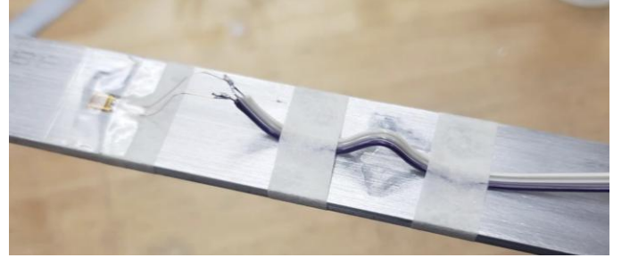
Fig. 3. The strain gauge was soldered to the connecting wires at the leads, and the connecting wire was taped with a hump for strain relief to avoid unnecessary stress on the sensitive wires while in use.
