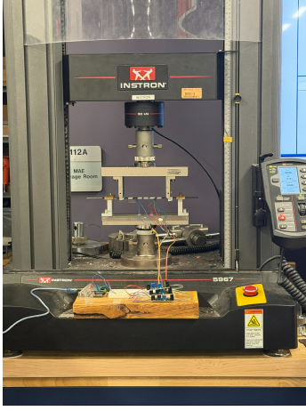
Fig. 11. Configuration of the carbon-fiber beam when implemented into the Instron UTM. The lower clamps keep the ends of the beam fixed, while the upper anvil applies an axial load to produce bending.
