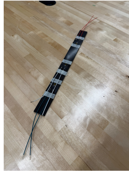
Fig. 7. Carbon fiber laminate sample prepared for four-point flexural testing. The sample features three surface-mounted strain gauges: one at the center and two equidistant from the center on opposite sides. Embedded electrical lead wires, with relief, extend from both ends to facilitate direct connection with Arduino.
