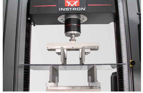
Fig. 5. Original setup for a four-point test on the carbon-fiber laminate sample. The sample is positioned across two lower support anvils and loaded by two upper loading anvils, utilizing an Instron universal testing machine [5].
